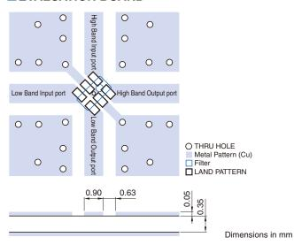
Line width to be designed to match  $50\Omega$  characteristic impedance, depending on PCB material and thickness.
