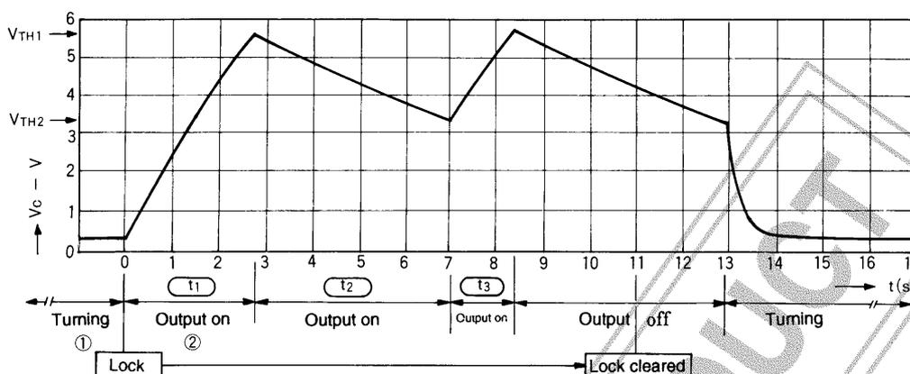
1. While the blades are turning, the capacitor is charged with a current of about  $3 \mu\text{A}$  (typical), and C is discharged by pulses that correspond to the motor speed.
