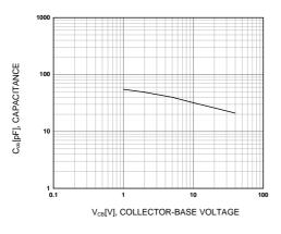
Figure 3. Collector Output Capacitance
