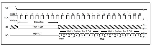
Figure 7-5. Read Status Register Instruction (QPI Mode)
