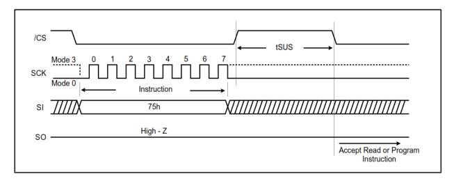
Figure 7-36. Erase Suspend instruction (QPI Mode)
