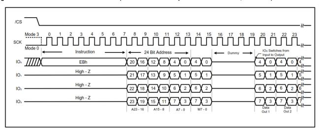
Figure 7-20. Fast Read Quad I/O Instruction (previous M7-0 = Axh, SPI mode)
