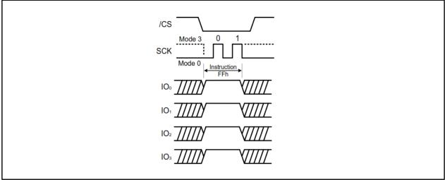
Figure 7-53. Word Read Quad I/O instruction (Previous instruction set M7-0= Axh, SPI Mode)
