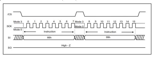
Figure 7-60. Enable Reset and Reset Instruction (QPI Mode)
