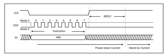
Figure 7-42. Release Power Down Instruction (QPI Mode)
