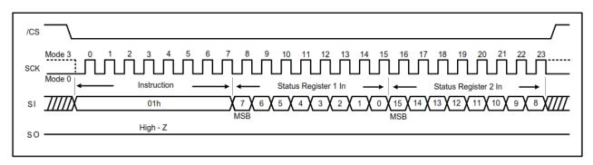
Figure 7-7. Write Status Register Instruction (QPI Mode)
