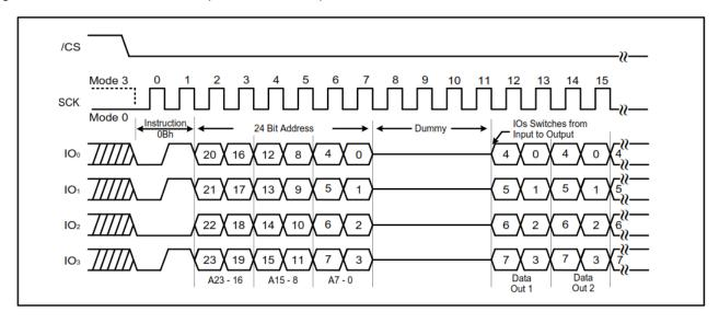
Figure 7-13. Fast Read instruction (QPI Mode, 104MHz)
