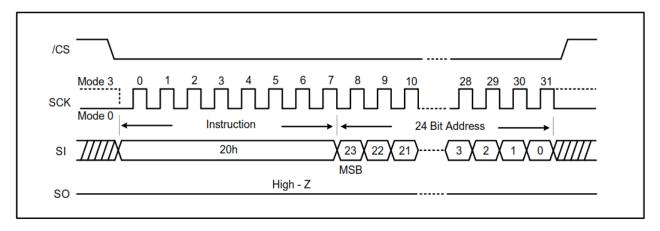
Figure 7-29. Block Erase Instruction (QPI Mode)
