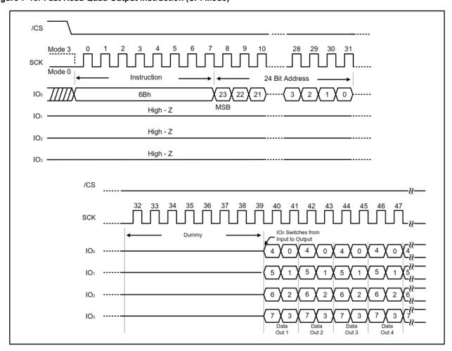
Figure 7-16. Fast Read Quad Output instruction (SPI Mode)
