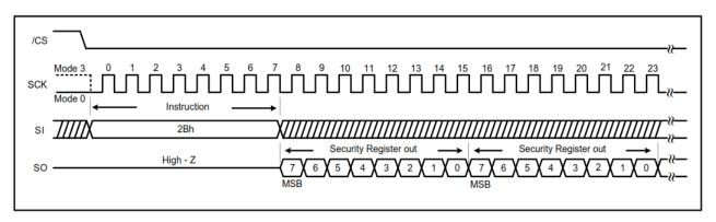
Figure 7-65. Read Security Register instruction (QPI Mode)
