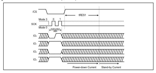
Figure 7-43. Release Power Down / Device ID Instruction (SPI Mode)
