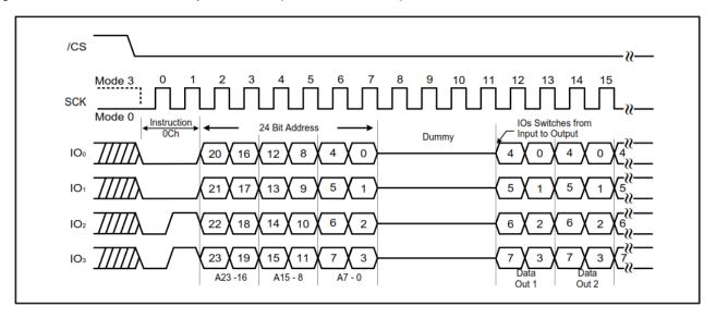
Figure 7-57. Burst Read with Wrap instruction (QPI Mode, 133MHz)\*
