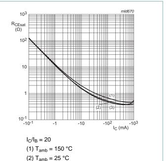
Fig 9. Collector-emitter equivalent on-resistance as a function of collector current; typical values
