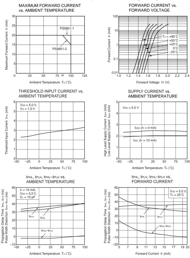
TYPICAL CHARACTERISTICS ( $T_A = 25^{\circ}C$ , unless otherwise specified)
